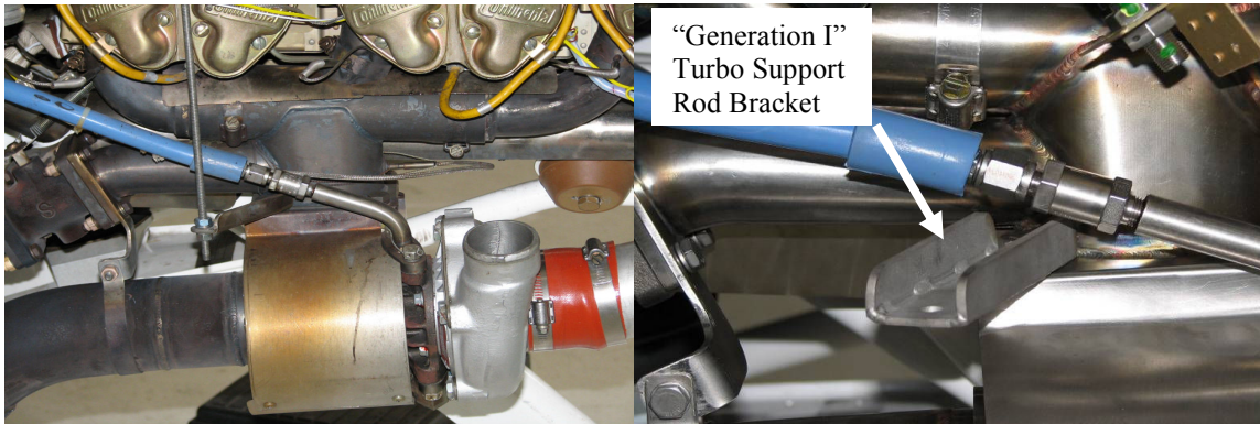
“Generation I” exhaust with bridge style turbo support rod bracket. Rod not shown in second picture.
